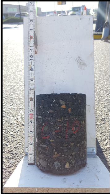
Core: 10 HMA: 6.3 in Soil: SM AB: 10.0 in
