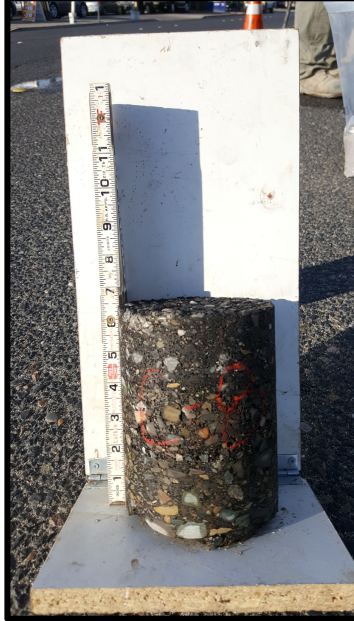
Core: 8 HMA: 6.5 in Soil: SM AB: 8.5 in
