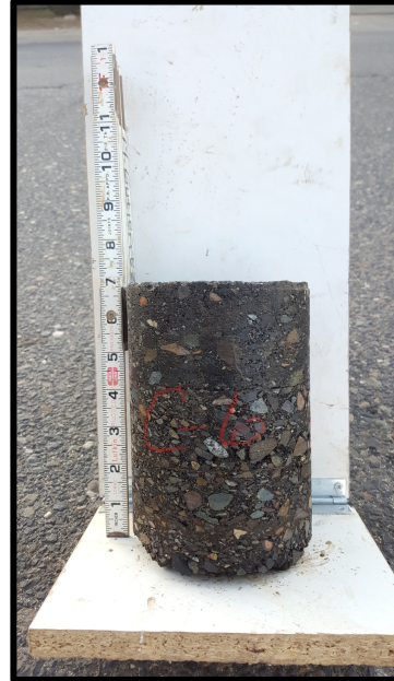
Core: 6 HMA: 6.8 in Soil: SM AB: 6.8 in
