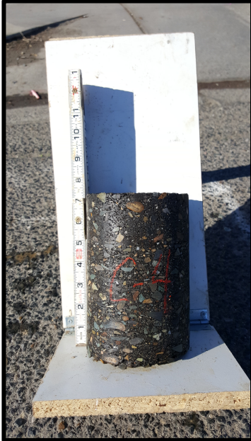
Core: 4 HMA: 7.3 in Soil: SM AB: 30.5 in
