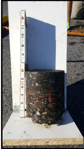
Core: 5 HMA: 6.0 in Soil: SM AB: 7.0 in
