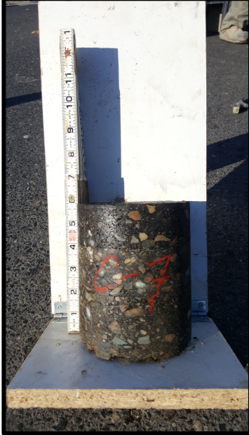
Core: 7 HMA: 5.8 in Soil: SM AB: 6.3 in
