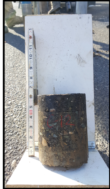
Core: 12 HMA: 6.0 in Soil: SM AB: 7.0 in
