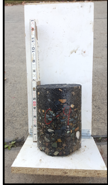
Core: 9 HMA: 6.3 in Soil: SM AB: 6.8 in
