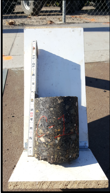
Core: 1 HMA: 6 in Soil: SM AB: 8 in
