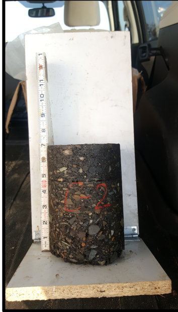
Core: 2 HMA: 6.8 in Soil: SM AB: 5.3 in
