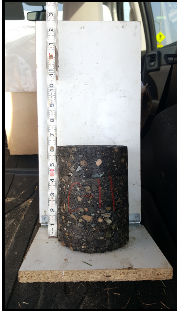
Core: 11 HMA: 6.1 in Soil: SM AB: 9.9 in
