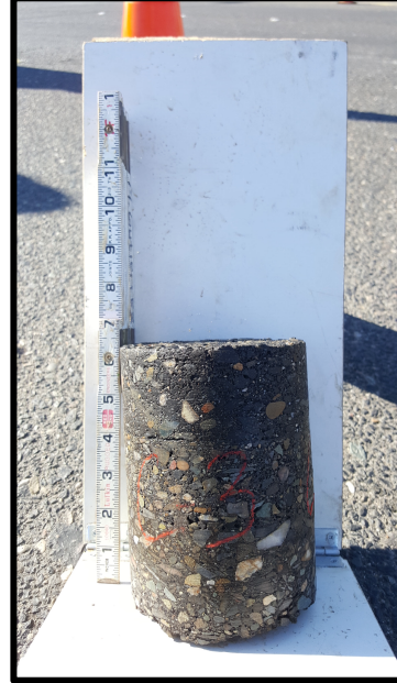
Core: 3 HMA: 6.3 in Soil: SM AB: 5.8 in
