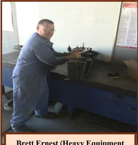
**Brett Ernest (Heavy Equipment Mechanic)** working on an air conditioning evaporator case
