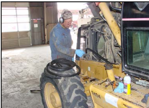
Ed Soares replacing a hydraulic line
