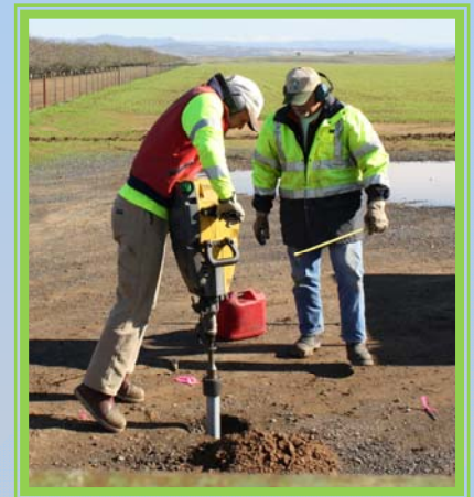
Scotty drives a 4-foot iron pipe through the hardpan layer.
