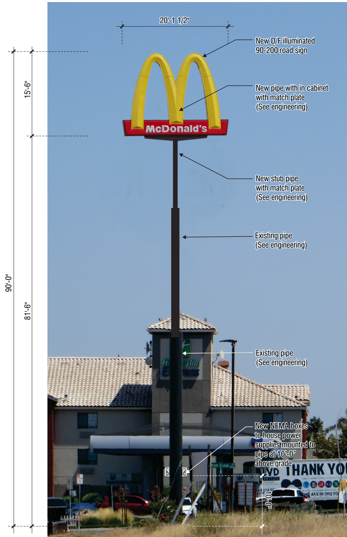
2 PROPOSED NEW D/F ILLUMINATED 90-200 ROAD ON EXISTING PIPE & INCREASE HEIGHT Approximate Scale: 3/32" = 1'-0"
