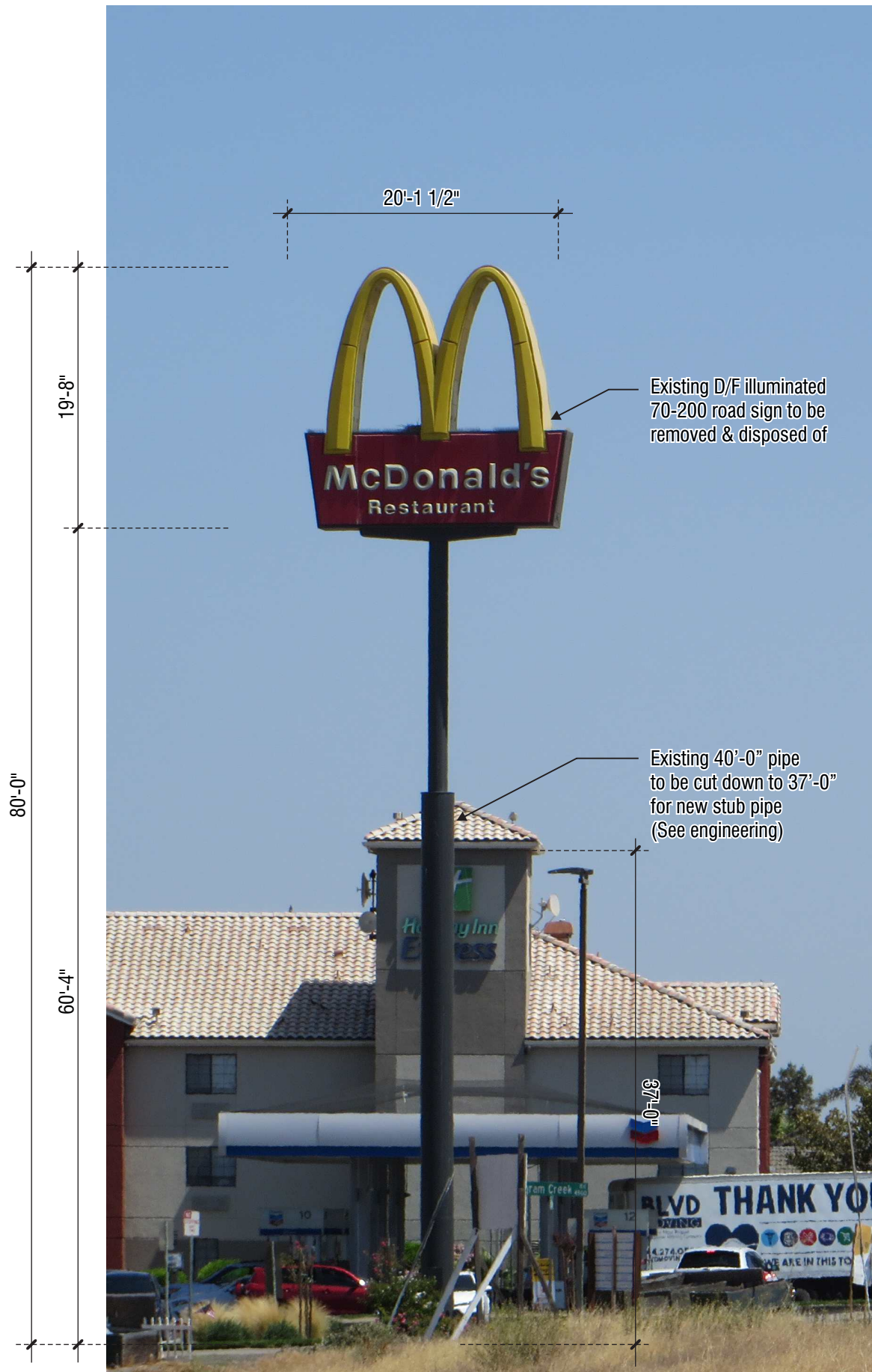
1 EXISTING D/F ILLUMINATED 70-200 ROAD SIGN Approximate Scale: 3/32" = 1'-0"
