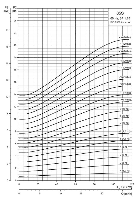
85S (85 gpm) pump power requirement (P2)
