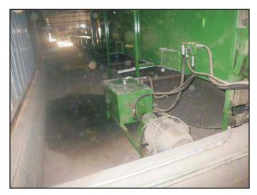
Photo 11: Hydraulic oil leak at packing machinery.
