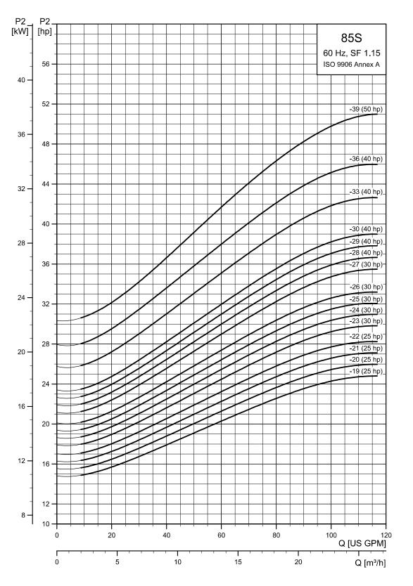
85S (85 gpm) pump power requirement (P2)
