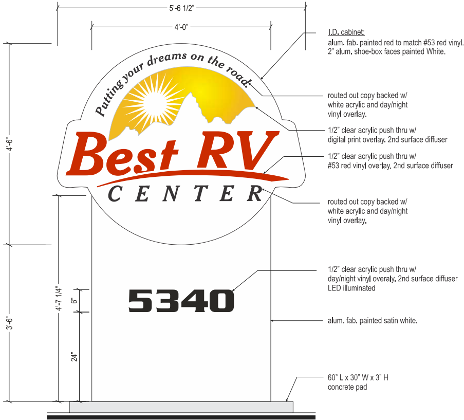
SIGN-M1: D/F LED ILLUMINATED MONUMENT SIGN Scale: 3/4" = 1'-0"
