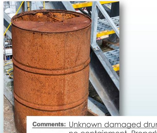
Comments: Unknown damaged drum, missing labels and no containment. Properly dispose of contents and drum ASAP.
