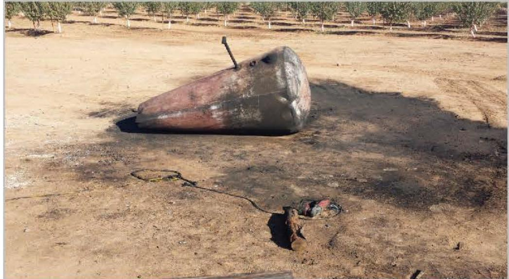
*"Damaged tank from explosion: Tank ends are bowed outward. No emergency venting evident. Small grinder with wire brush wheel nearby."—Hank Moore, Merced County Fire Marshal*
