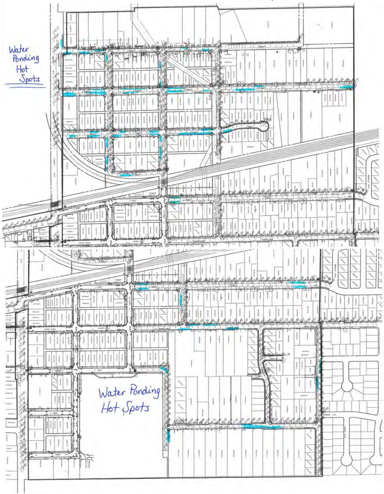
Figure 17A: Areas of Ponding Water after Major Rain Events (Hot Spots) Areas North of Yosemite Blvd Phase 1A, 2, 3)
