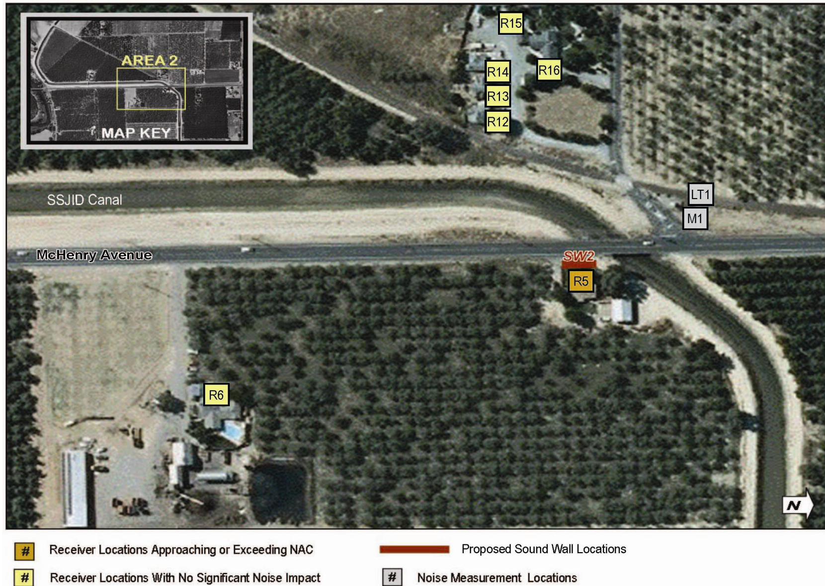
Figure 2-11 Receptor & Potential Sound Wall Locations (Area 2)
