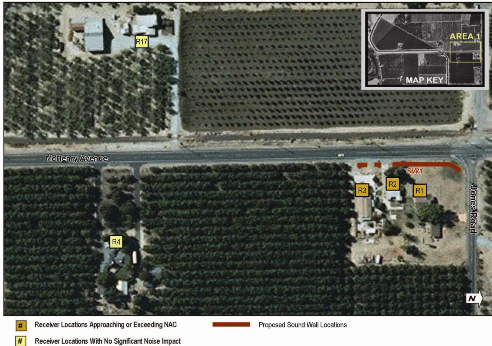
Figure 2-10 Receptor & Potential Sound Wall Locations (Area 1)
