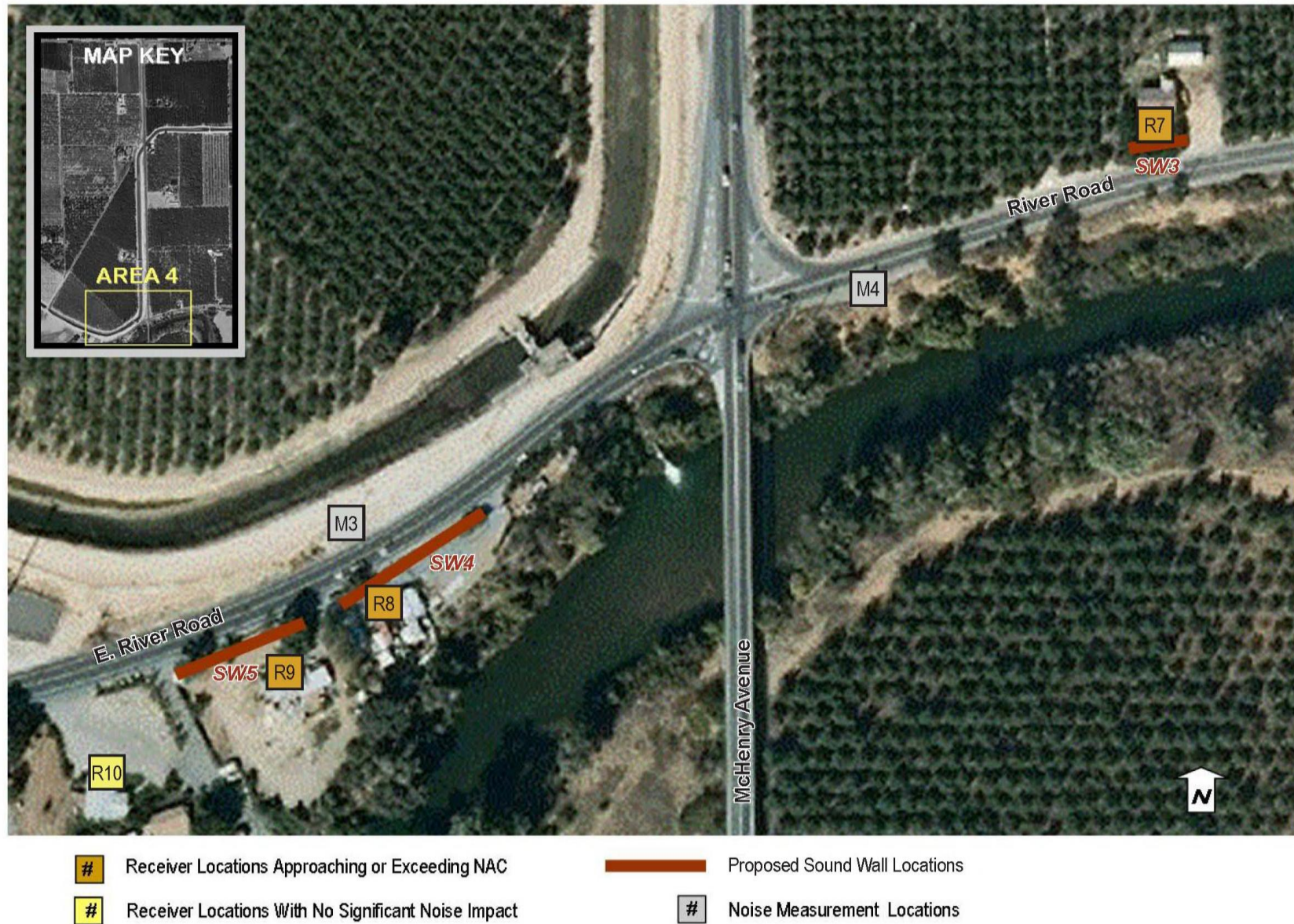
Figure 2-13 Receptor & Potential Sound Wall Locations (Area 4)
