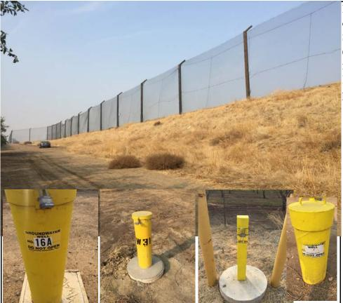
Photograph 7 - Northern boundary of subject property: Fink Landfill. Select monitoring wells shown (well 16, 20, 24 and 31). Several monitoring wells were inside the landfill boundary line, as shown in photograph 8.
