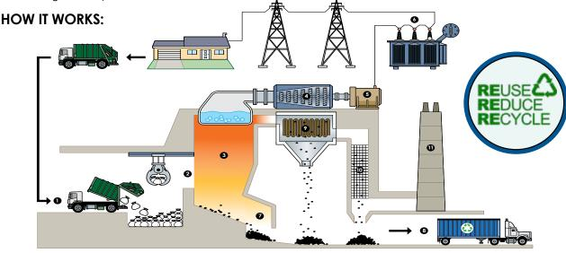
1 Waste is delivered to the facility and stored in a bunker.
