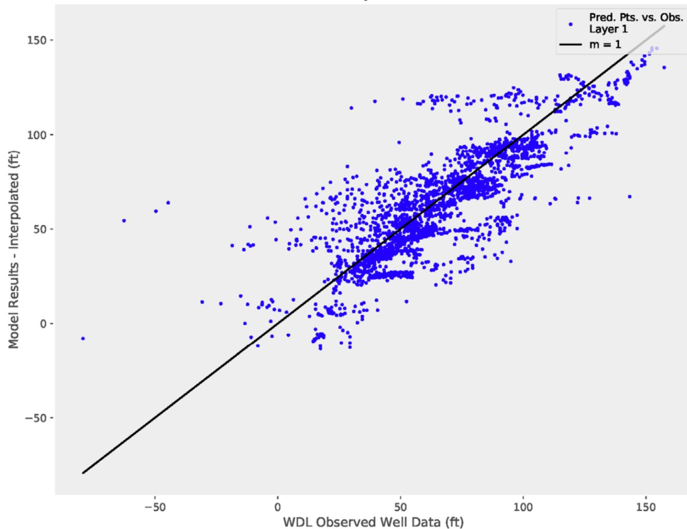
Interpolated Model Results (2000-2015) vs. WDL Observed Well Data
