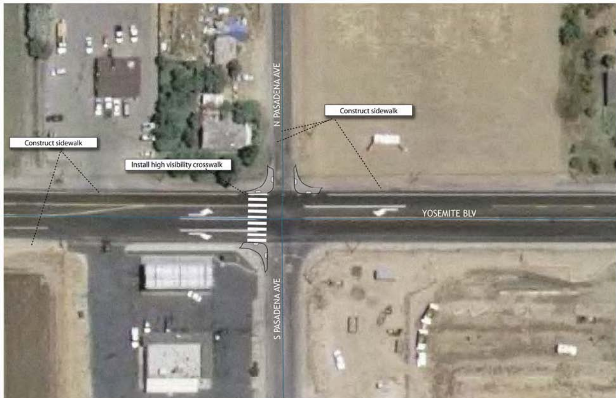
YOSEMITE BLVD AND PASADENA AVE INTERSECTION IMPROVEMENTS
