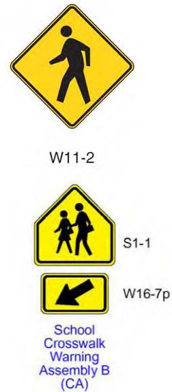
Figure B-20: Pedestrian Warning Signage
